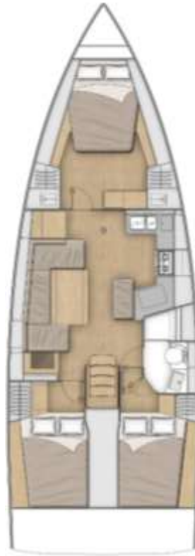
3C 1H + optional washbasin furniture in forward cabin. Also available with the 2C1T layout
